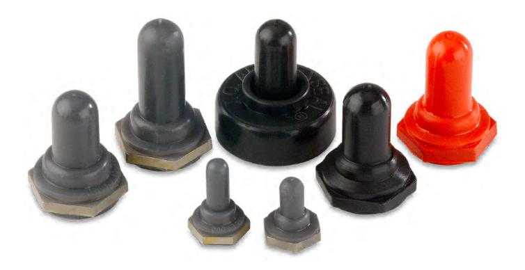
Toggle switches are one of the most popular forms of switches due to their simple back-and-forth actuation. <u>Toggle boots</u> are protective covers for this switch type, also referred to as a toggle bat, consisting of a single-component impermeable outer silicone seal, a molded-in threaded mounting nut of nickel or brass, and a panel-sealing rib.
