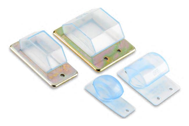
Contamination within lever-actuated circuit breakers can cause short circuits and fires. With mission-critical functionality, these levers require durable seals for harsh environmental conditions. APM Hexseal offers both front- and back-of-panel boot styles with a sealing rib that runs the circumference of the flange's underside for a high-quality seal.
