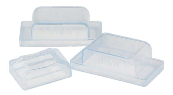
A rocker switch is a seesaw-like switch with on/off capabilities. <u>Rocker boots</u> will not feature a threaded mounting nut, frame, or insert, as rocker switches do not use a threaded mounting bushing. We design them so that installers can mount them on the rocker switch before they install the switch itself. Transparent silicone construction allows operators to easily view the switch position.
